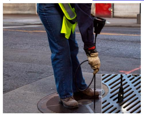
The FLIR VS290-32 videoscope combines thermal imaging and a visible camera on a replaceable, two-meter-long probe for safer and more efficient inspections of vented manholes without having to remove the cover. (Photo: Business Wire)
