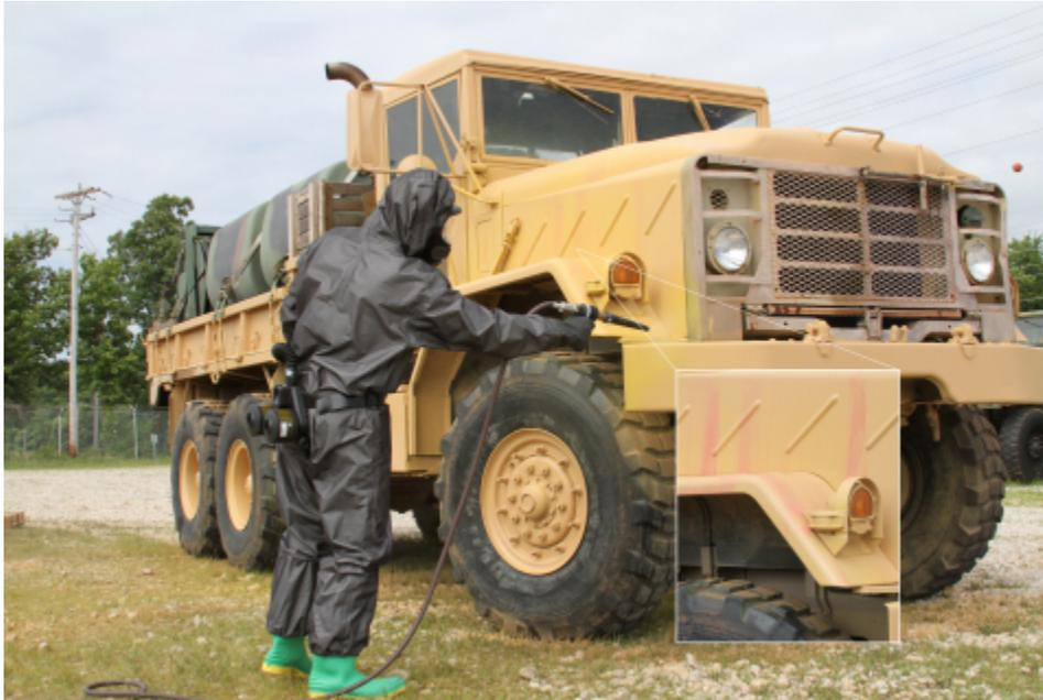
FLIR Agentase C2 spray quickly changes color on a surface if a chemical warfare agent is present. With faster and more targeted detection, military decontamination experts can locate trace levels of contamination and precisely mitigate the threat.
