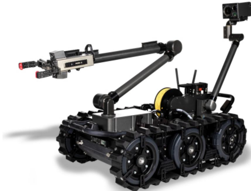
Explosive Ordnance Disposal (EOD) teams use the FLIR Centaur unmanned ground system to assist in disarming landmines, unexploded ordnance, improvised explosive devices, and similar dangerous tasks. Operators can quickly attach different sensors and payloads to the robot to address other missions, including chemical, biological, radiological and nuclear (CBRN) threats.
