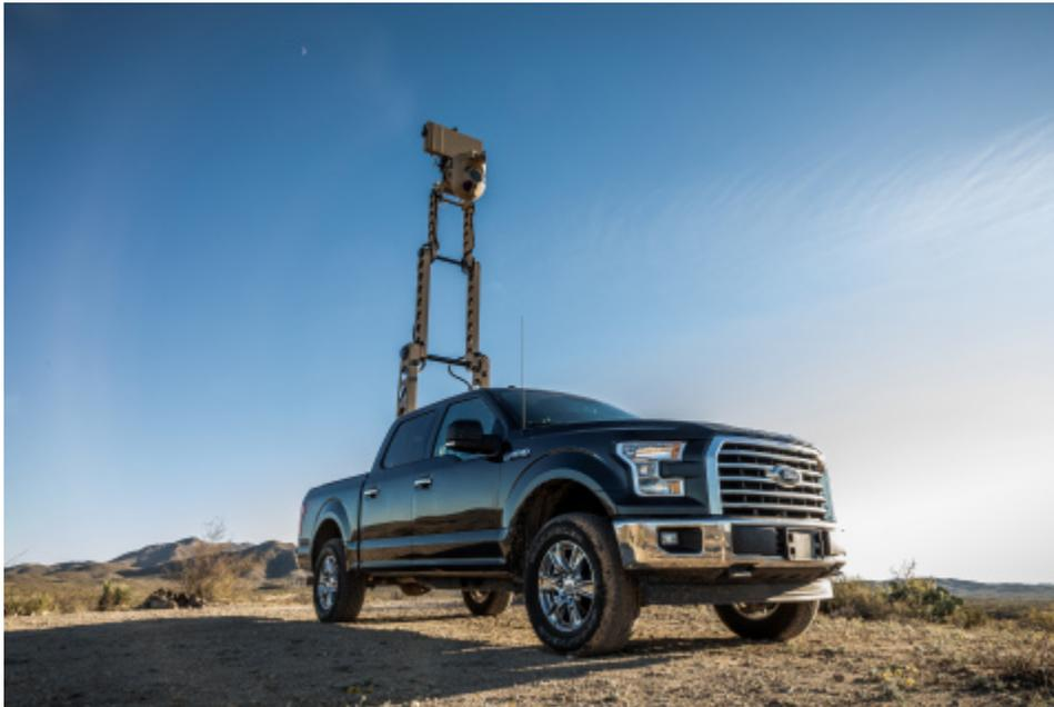
The FLIR LVSS™ provides the most advanced, integrated surveillance available that can track up to 500 objects at once at ranges greater than 10 miles (16 km). LVSS is well suited to missions that call for speed, mobility and flexibility, including protecting remote borders, shorelines, and forward operating bases. A single operator can deploy and operate the system's 16-foot mast from the cab of a pickup truck in less than 30 seconds. (Photo: Business Wire)
