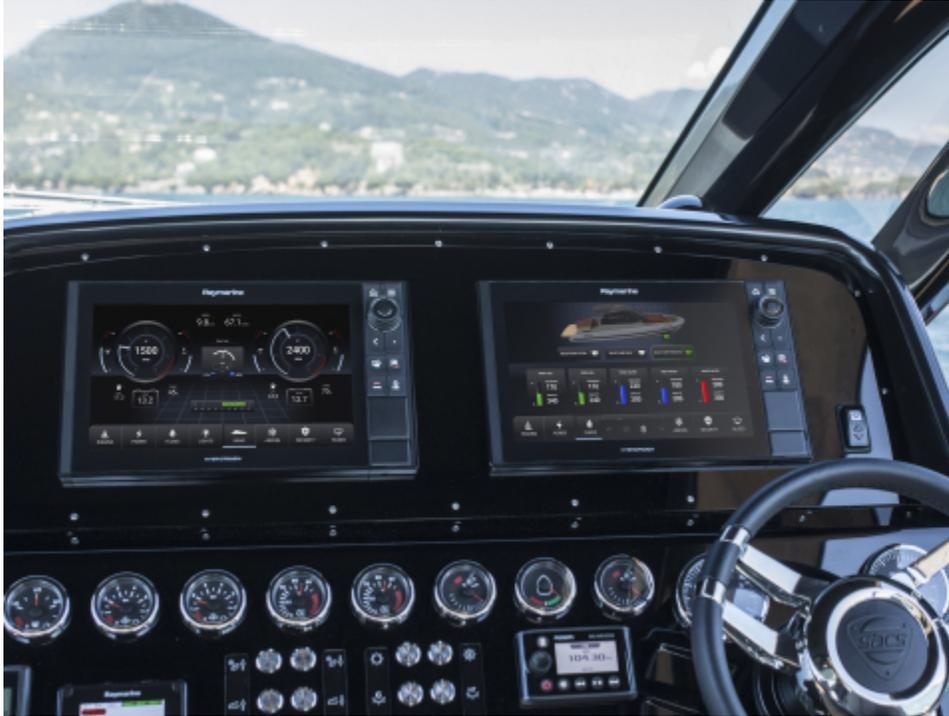
Raymarine YachtSense technology brings home automation-like capabilities to luxury boats by replacing physical switches with touch screens controls integrated into Raymarine's Axiom marine navigation systems. (Photo: Business Wire)
