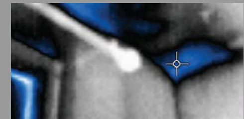
IGM shows cold spots, guiding where to measure
