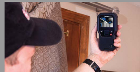
Scanning ceiling &amp; wall joint for moisture issues
