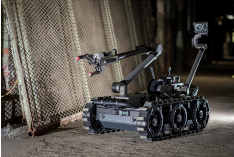
U.S. military explosive ordnance disposal (EOD) teams will use the FLIR Centaur™ ground robot to help disarm improvised explosive devices, unexploded ordnance, and perform similar hazardous tasks. Operators can quickly attach different sensors and payloads to the advanced 160-pound robot to support other functions, including chemical, biological, radiological and nuclear (CBRN) missions. (Photo: Business Wire)
