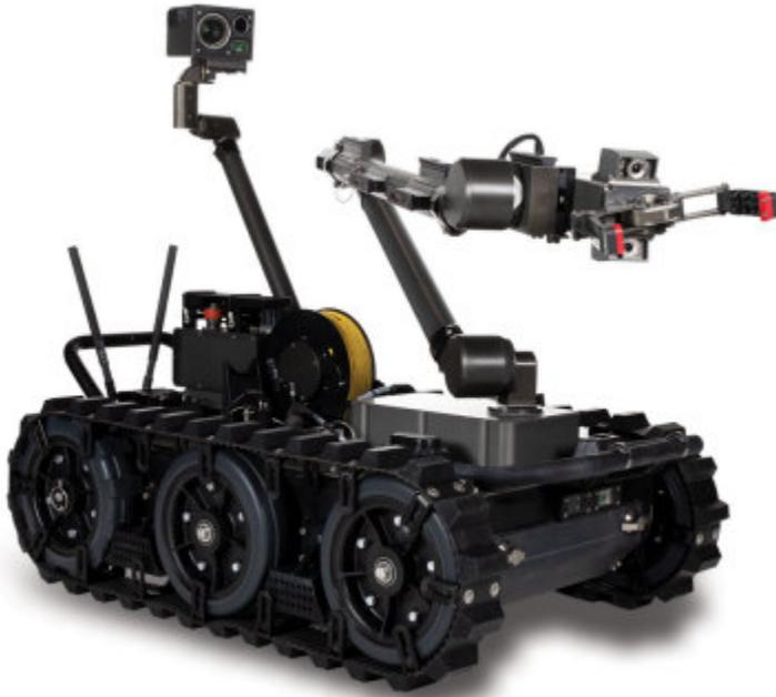
U.S. Marine Corps teams will use the FLIR Centaur™ robot to help disarm improvised explosive devices, unexploded ordnance, and perform similar hazardous tasks. Different sensors and payloads can be added to the 160-lb. Centaur to support a range of missions. (Photo: Business Wire)
