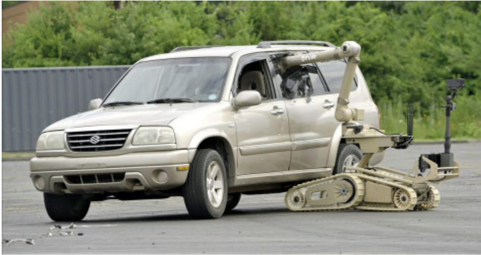
The CRS-H program will give the Army a 'program of record' to build and sustain a fleet of large UGVs for years to come. The CRS-H platform calls for a robot weighing up to 700 pounds. Army Explosive Ordnance Disposal (EOD) units will use the system to perform a range of missions, such as disarming vehicle-borne improvised explosive devices (VBIEDs), unexploded ordnance, or related heavy-duty tasks. A variety of sensors and payloads also can be added to the UGV to support other missions.
