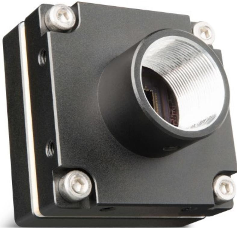
Traditional rules-based software is ideal for straightforward tasks such as barcode reading or checking a manufactured part against specifications. The FLIR Firefly combines a new, affordable machine vision platform with the power of deep learning to address complex and subjective problems such as recognizing faces or classifying the quality of a solar panel.
