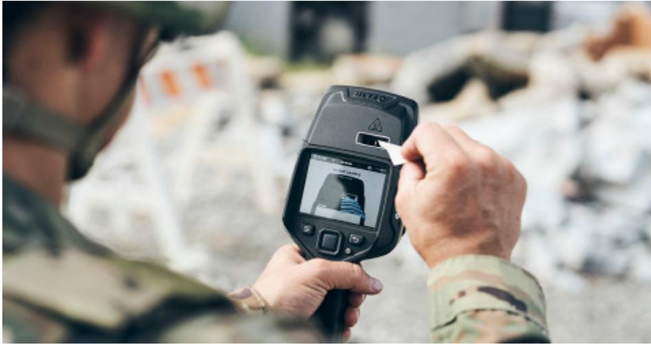
FLIR Systems' TrueTrace® detection technology features a new five-channel sensor array that delivers expanded threat coverage. TrueTrace can accurately detect a wide range of explosives at nanogram to sub-nanogram levels – including military, commercial, improvised, and homemade explosives – allowing users to gain actionable intelligence through identification of threats in as little as ten seconds.
